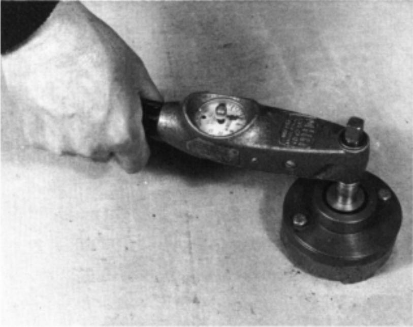
**Figure 4.17** Torquemeter loading method.
