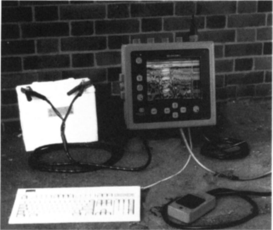
**Figure 8.4** Digital impulse radar system.
