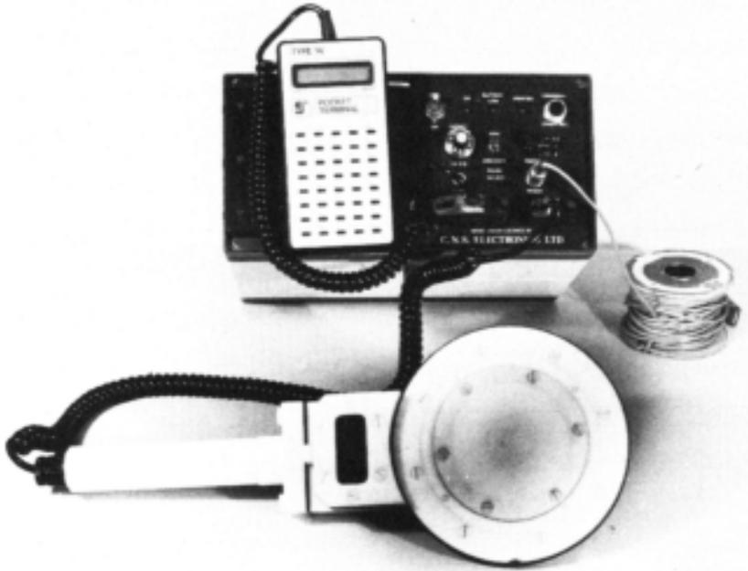
**Figure 7.9** 'Wheel' half-cell equipment.
