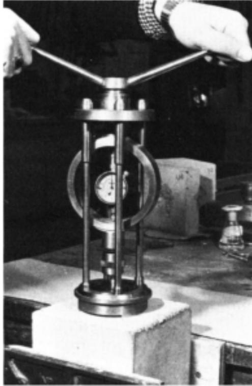
**Figure 4.18** Proving ring loading method.
