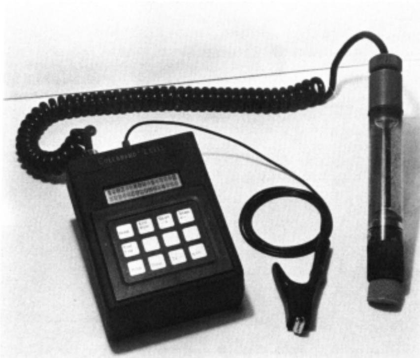
**Figure 7.8** Single half-cell instrumentation.
