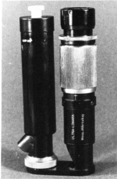
**Figure 6.10** Crack microscope.
