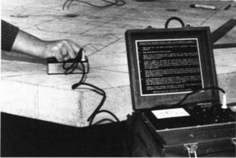
**Figure 7.3** Typical simple covermeter.
