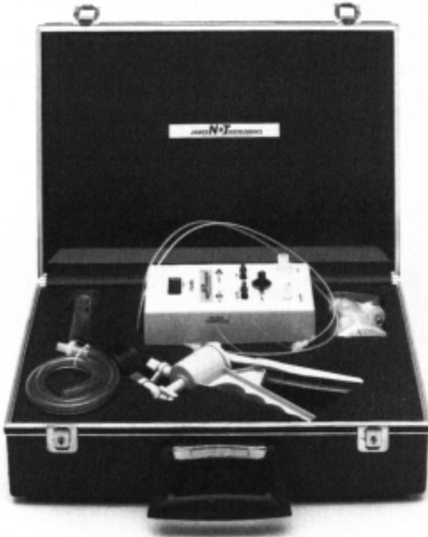
**Figure 7.19** Automatic Figg test equipment (photograph by courtesy of James Instruments Inc).
