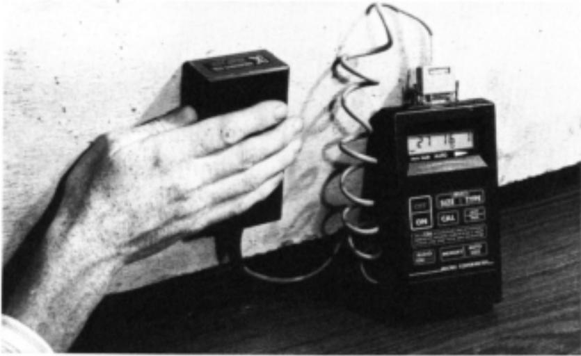
**Figure 7.5** Microcovermeter.
