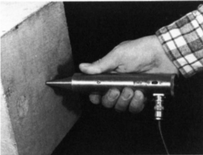
**Figure 3.3** Exponential probe transducer.
